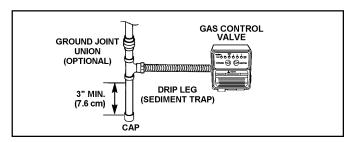
FIGURE 12. GAS PIPING WITH FLEXIBLE CONNECTOR.
